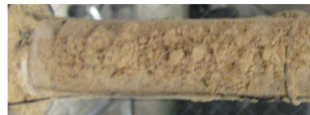
Ash on surface of OTM tube
