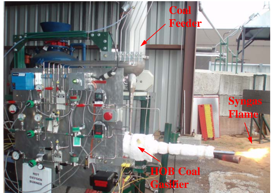
Praxair Hot Oxygen Burner for Coal Syngas
